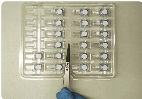
3. Remove the modules from the blister using plastic tweezers
