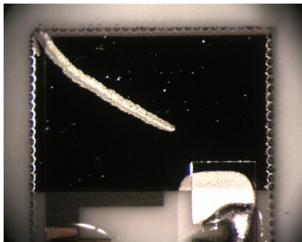
Picture 8: Sensor with a scratch
